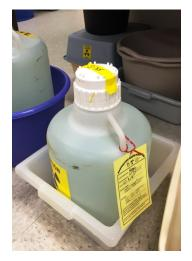
**Radioactive Liquids**: Containers holding radioactive liquids are decanted into a thick-walled plastic carboy (jug) issued by EHS. Carboys are marked with the name of the radionuclide that may be placed inside it. Labs are issued a separate liquid carboy for each radionuclide in use. All radioactive liquid carboys must be stored inside a secondary container in case of leakage.
